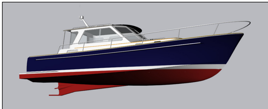
The skag adds stability in a seaway while protecting the running gear
